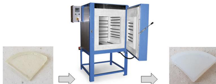
Figure 9 - Glass ceramic synthesis sketch.
