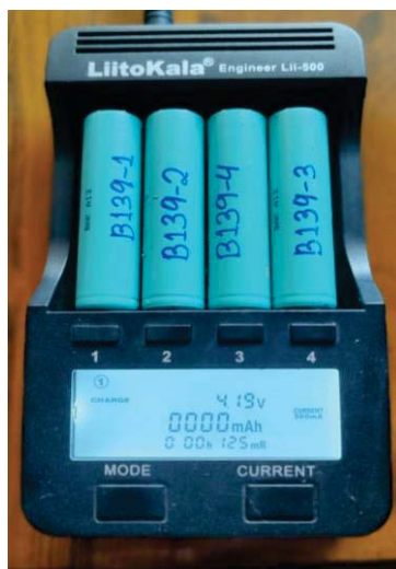
Figure 6: LiitoKala smart charger Engineer LII-500 testing a set of cells.
