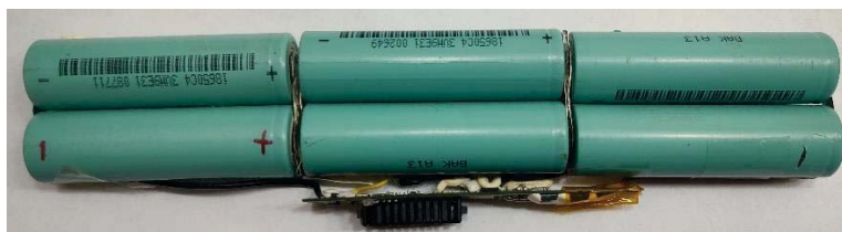
Figure 4: Inside the battery in Fig. (3) before the cells were separated.
