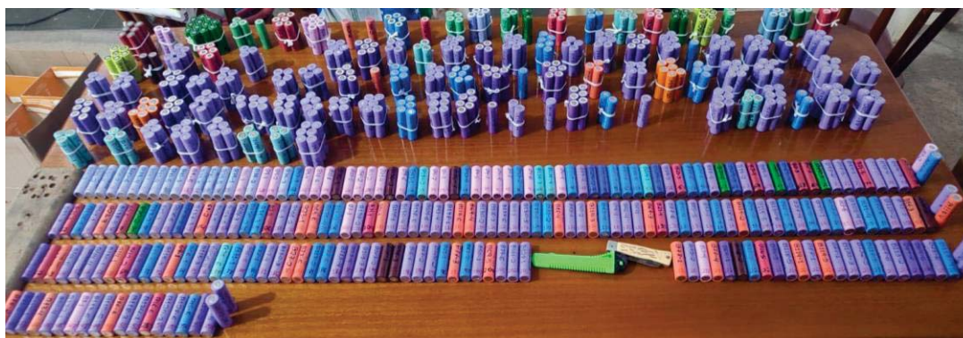
Figure 5: Batteries of cells being separated and cataloged after dismantling and treating laptop batteries.
