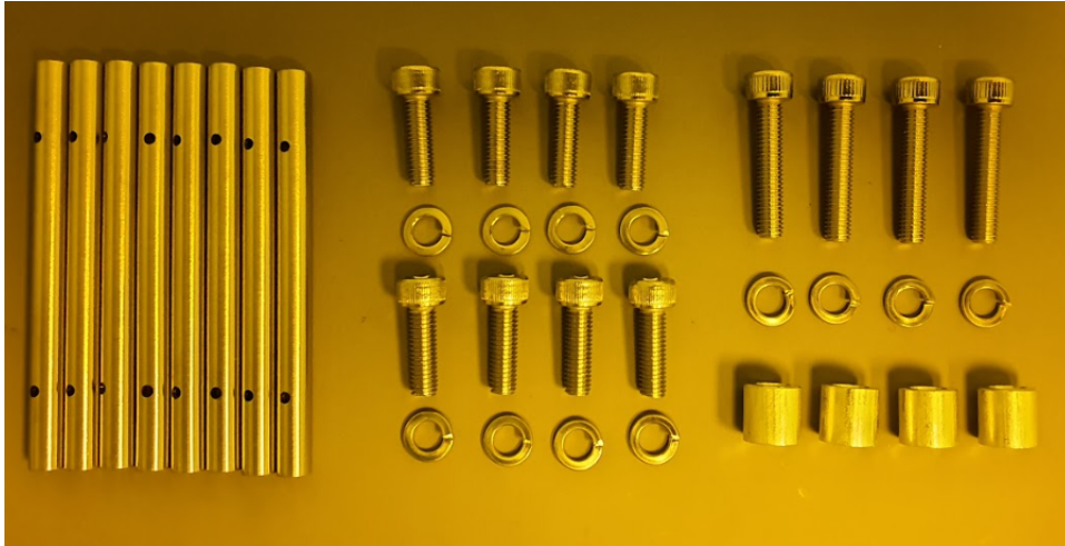
Figure 15 – A set of 8x Standoffs and all the M5 screws washers and spacers for mounting one set wit a pair of X-Arapucas.
