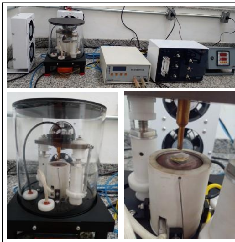
Figure VII-16 - Thermal Poling assembly at UNIFAL-MG (Brazil).
